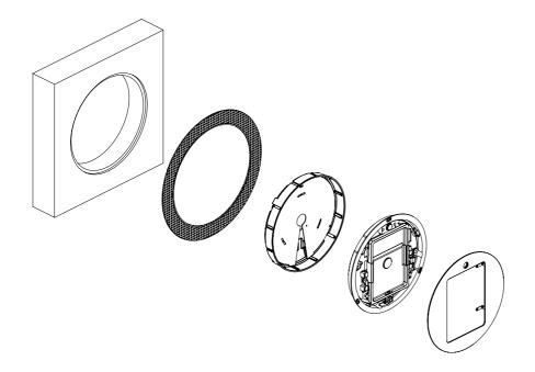
Install the flush box so deep that it rests firmly on the inner ring of the frame.
