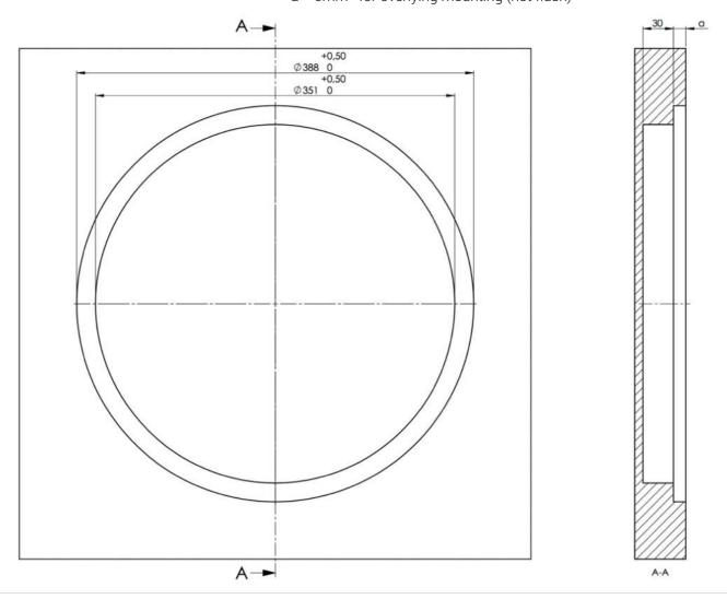
a = 9mm for flush-mounted installation a = 0mm for overlying mounting (not flush)
