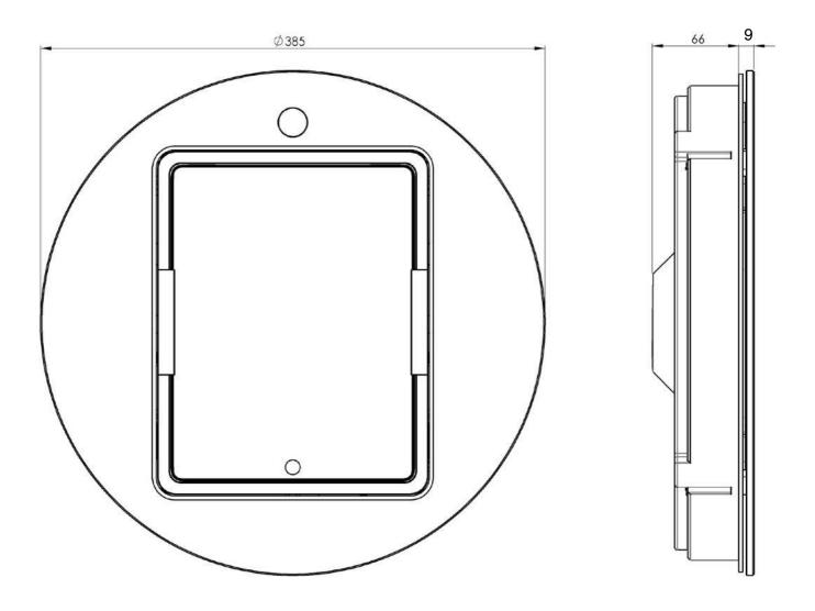
Installation Use the three <u>inner</u> holes to screw the mounting plate to the wall!
