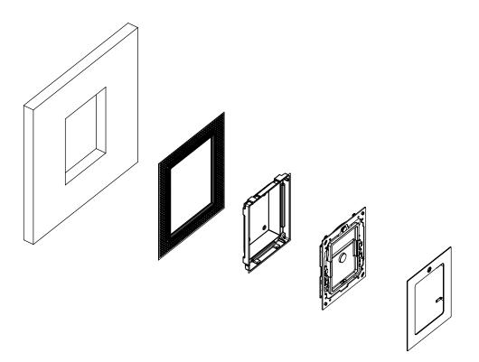
Install the flush box so deep that it rests firmly on the inner ring of the frame.
