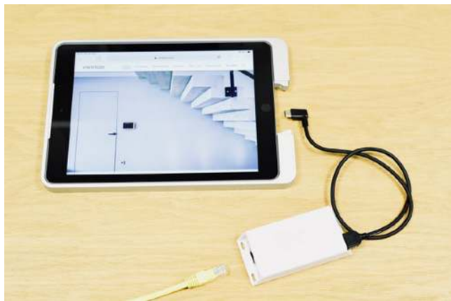
PoE Splitter for iPads with USB-C connector.
