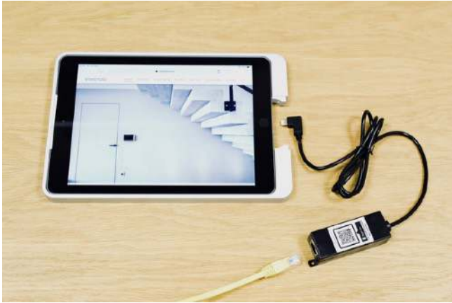
PoE Splitter for iPads with Lightning connector.
