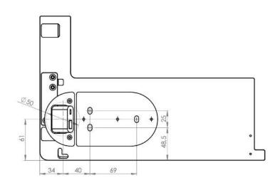
back view ! Attention: Measurements show free for iPad mini 4. Measurements for other generation on following page. The size of free varies depending on the iPad generation. Mounting plate is always the same, it allows you to change iPad generation easily.
